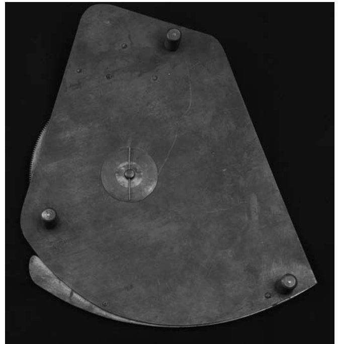
Fig. 5 (a) Rambaut's mechanical device for finding solutions to Kepler's Equation - fecit Henry Minn c.1905/6. (b) Reverse side of Rambaut's instrument. Museum of the History of Science inventory number 11031. Photographs by Richard Rowley.
