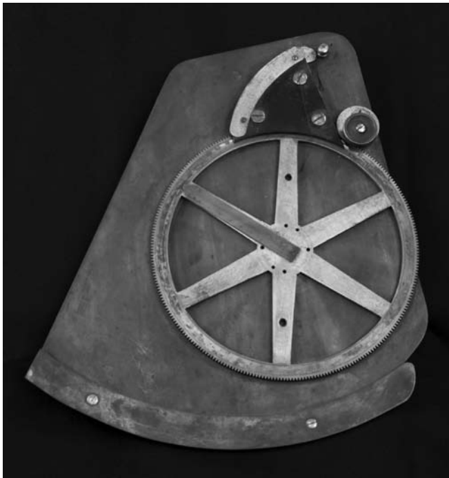
Fig. 5 (a) Rambaut's mechanical device for finding solutions to Kepler's Equation - fecit Henry Minn c.1905/6. (b) Reverse side of Rambaut's instrument. Museum of the History of Science inventory number 11031. Photographs by Richard Rowley.
