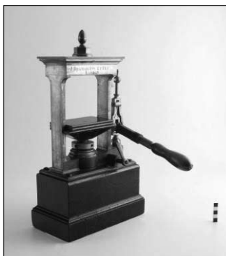
Fig. 5 Faraday's hydraulic press at the Royal Institution. (Photograph courtesy of the Royal Institution.)
